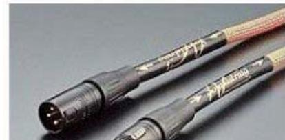
The ground connection is achieved by crimping and the center conductor is attached with a drop of solder. The pin is gold plated copper. It is slightly elongated and the tip is wider than the shaft. The connector is fitted with a 24Kt gold plated, beryllium copper element, and a finely cured wood housing screws into the back of the connector to minimize resonance.
